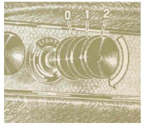
Turning the headlight switch knob can regulate the intensity of the instrument lighting. The further the knob is turned in a clockwise direction, the stronger the instrument lighting will be.
